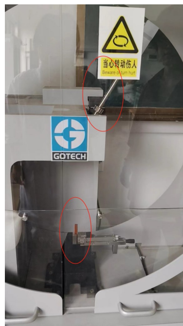
图4 简支梁法测试冲击强度 Fig.4 Impact strength test using simply supported beam method
